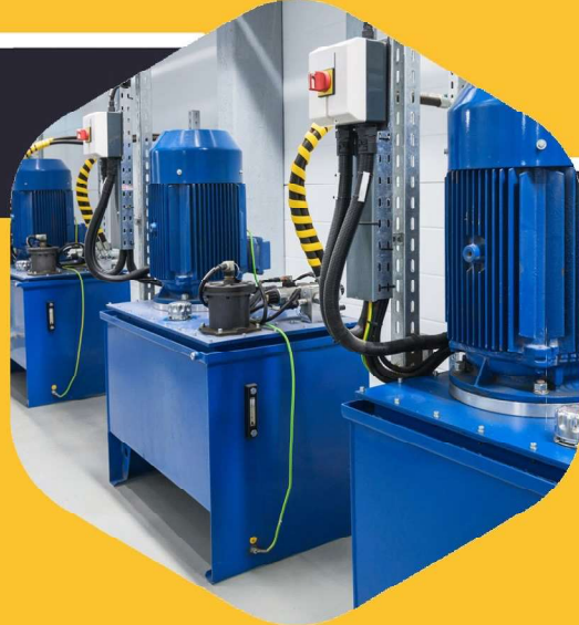
Hydraulic Power Unit
